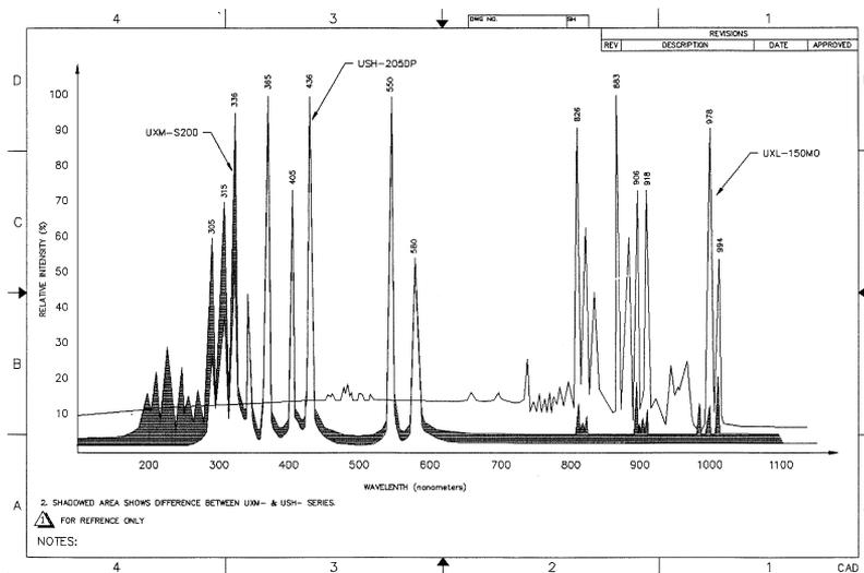
**Figure 2** Relative intensities of HBO, XBO, and combined XBO/HBO arcs. In comparison, the spectrum for an incandescent halogen lamp would run along the baseline. (Courtesy of Ushio America, Inc., Cerritos, CA.)
