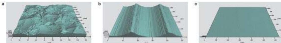
Figure 7 - Changes in metal surface during processing: a) prior to machining,  $RSa = 18.853 \mu\text{m}$ ; b) after turning,  $RSa = 5.543 \mu\text{m}$ ; and c) after final polish,  $RSa = 0.034 \mu\text{m}$ . (Images courtesy of **Carl Zeiss, Inc.**)
