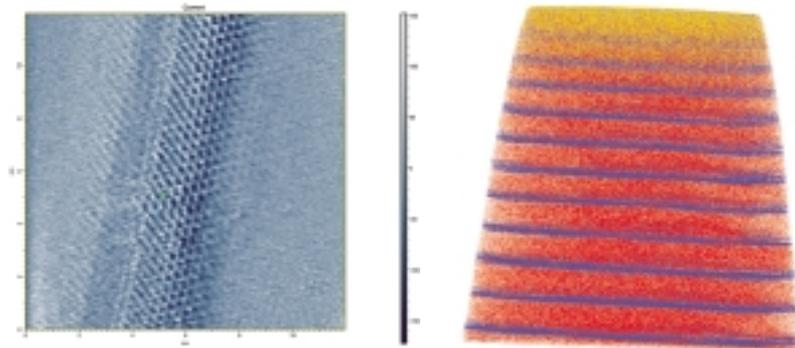
*Figure 6* Atomic level imaging. Left: Structure detail of a carbon nanotube taken with a scanning probe microscope. (Image courtesy of **NT-MDT**, Moscow, Russia.) Right: Multilayered Pt Mn Ga nanofilm taken with local electrode atom probe (LEAP). (Image courtesy of **Imago**, Madison, WI.)
