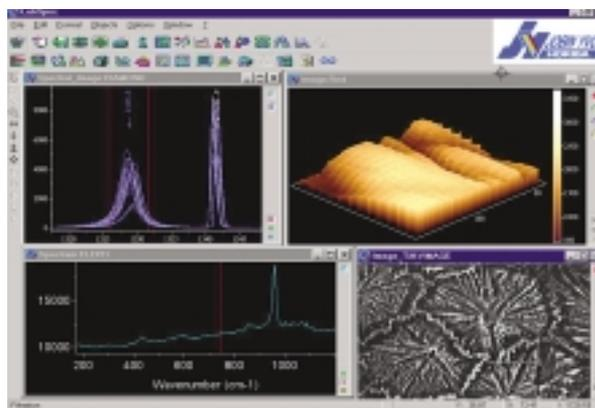
**Figure 2** Clockwise from lower left: single-line Raman spectrum, overlaid Raman spectra, Raman map, and brightfield microscopy image; objective magnification:  $50\times$ . (Image courtesy of Jobin Yvon.)
