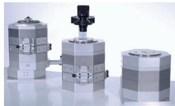
Figure 2 **TILL Photonics's** flexible, automated, space-age iMIC offers multiple ports for cameras and light sources and programmable user profiles. From left to right: a) DiChrotome configuration for dual-emission fluorescence and FRET experiments, b) more traditional inverted microscopy configuration with conventional condenser and transmitted light illumination, and c) core module for fluorescence and light microscopy. (Image courtesy of **Agilent** and **TILL Photonics**.)
