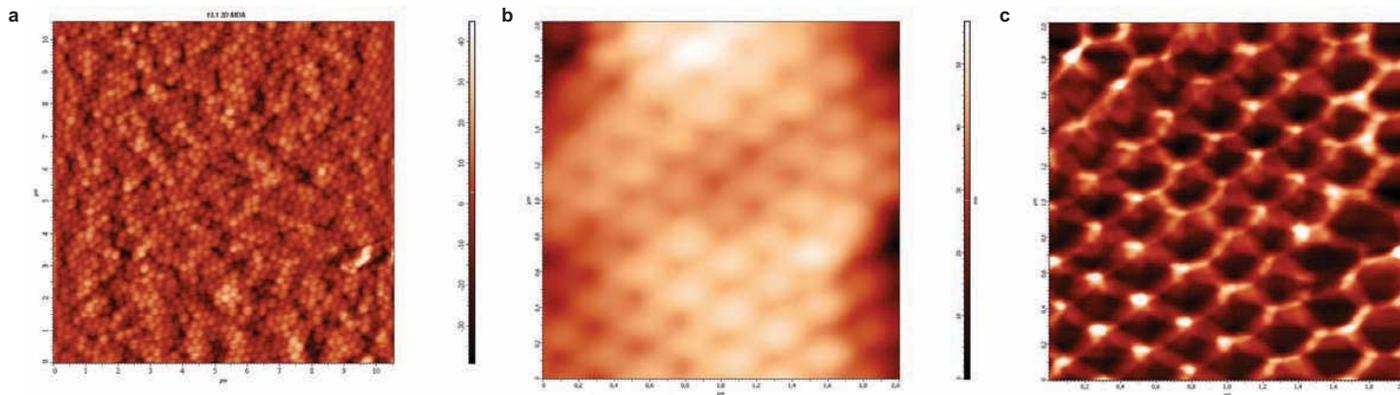
Figure 4 SolverNext delivers a wide range of conventional AFM/STM imaging modes. a) topography of latex:  $10 \mu\text{m} \times 10 \mu\text{m}$  scan, b) topography of latex:  $2 \mu\text{m} \times 2 \mu\text{m}$  scan, and c) phase image of latex:  $2 \mu\text{m} \times 2 \mu\text{m}$  scan.
