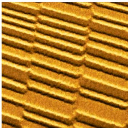
Figure 5 Magnetic force microscopy of a hard disk drive showing the magnetic bits and bytes.
