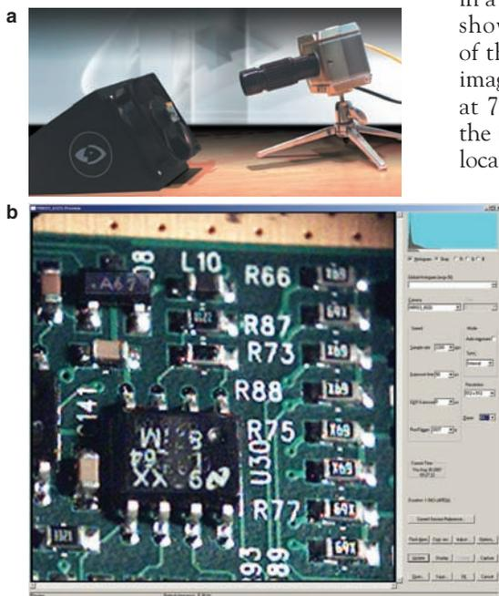
Figure 1 The Miro camera provides long working distances at high magnification coupled with fast action. a) Camera setup illustrating long working distance; b) image of parts taken at that distance, rotating at 7200 rpm. (Image courtesy of Vision Research.)
