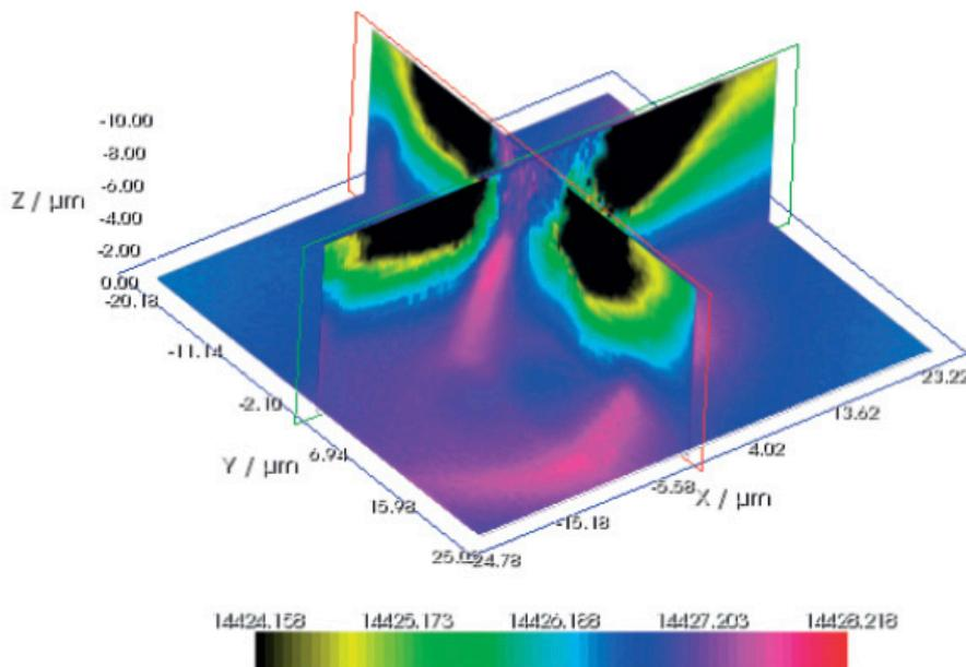
Figure 2 3-D imaging of stress within a ruby using **Renishaw's** new StreamLineHR.
