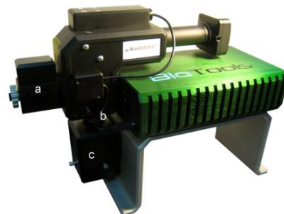
Figure 4 The new shoe-box-sized BioRAMAN from **BioTools** offers the flexibility of both a microscope and a cuvette system, and features sample holders for a) liquids, b) microscopy samples, and c) solids.
